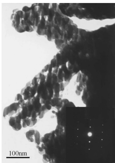
Figure 6 TEM image of MoN particles (prepared via heated precursor at 1073 K for 5 h).
