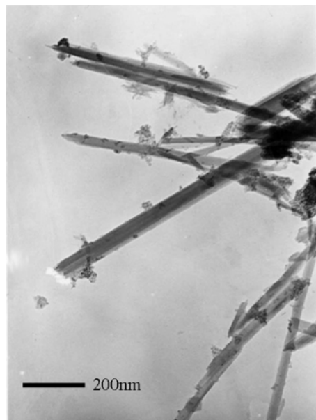
Figure 7 TEM image of MoN nanorods (prepared via \text{Al}_2\text{O}_3 /precursor at 953 K for 5 h).
